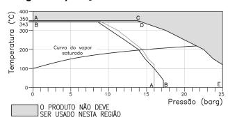
A-A: EN1092 PN16 B-B: ASME B16.42 150# A-C-E: EN1092 PN25 B-D-E: ASME B16.42 300#
